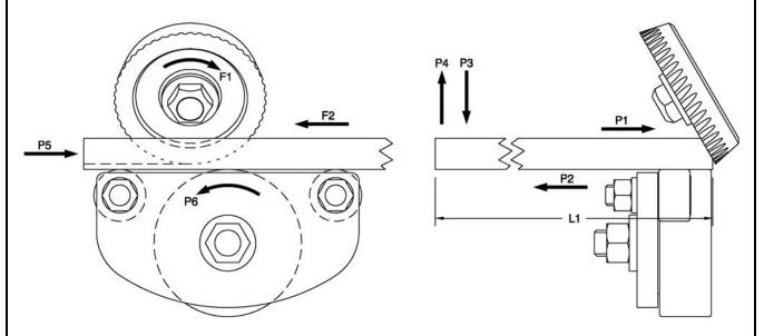
The rotary shearing cutter on the KBM<sub>®</sub>-18 Portable Plate Edge Bevelling Machine is subjected to considerable stress under load. The drawings above outline the dynamic forces that may be applied to a cutter in operation.
