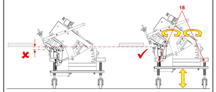
Using the hydraulic pump on the optional hydraulic lift undercarriage, adjust the working height of the machine to suit the height of the work table (the top of the Main Roller, after adjusting to desired bevel depth, is to be the same height as the underside of the plate to be bevelled). To lower the working height of the machine, slowly turn the release valve (located on the pump body) counter clockwise. Turn the valve clockwise once the desired height is reached
