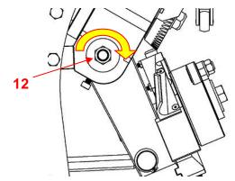
result in undesirable motion (forward or backwards, depending on the tilt angle) if it is not properly supported first. Slightly loosen the two (2) bolts, one (1) on each side of the Tilting Frame Base, so that there is still enough clamping tension to prevent undesirable tilting motion of the main body of the machine, but sufficient enough to allow the tilting angle to be manually positioned.
