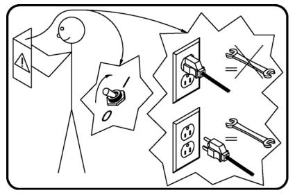
This label is attached to the Gullco bevelling machine and its intent is to instruct all those concerned to read the manual before operating the unit and before performing service, as well as to positively disconnect the unit from all power supplies before servicing.
