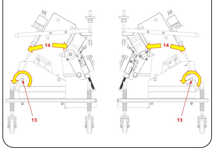
15. Re-tighten the two (2) bolts, one (1) on each side of the Tilting Frame Base.
