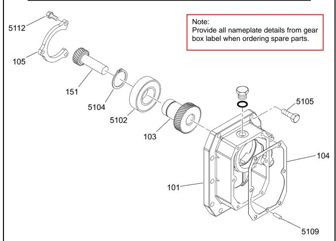
If component damage occurs, Gullco strongly recommends replacing the KBM-18-201 Gear Module Assembly, as it is more readily available and has been precision assembled & adjusted. Special tooling and procedures are required to rebuild these gear modules and should only be performed by qualified technicians.
