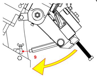
from both sides of the Cutter Shaft Housing to prevent the bolt from twisting. *Note: the alignment is the same for the 37.5° & 45° bevel angles.*
