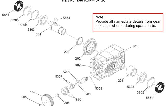
If component damage occurs, Gullco strongly recommends replacing the KBM-18-127 Gearbox Sub Assembly, as it is more readily available and has been precision assembled & adjusted. Special tooling and procedures are required to rebuild these gearboxes and therefore not recommended.
